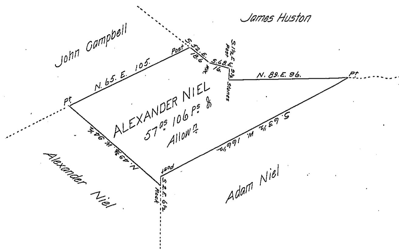
A Draught of a Tract of Land situate in Dickinson Township Cumberland County containing 57<sup>9</sup>/<sub>16</sub> 106 P<sup>s</sup> and allowance of six P. Cent for Roads &c. It being part of a larger tract of 158<sup>9</sup>/<sub>16</sub> 60 P<sup>s</sup> and allow. Surveyed in pursuance of a warrant granted to Alexander Niel Dated the 28<sup>th</sup> November 1771. Resurveyed & Divided the 17<sup>th</sup> Day of February A.D. 1807.
